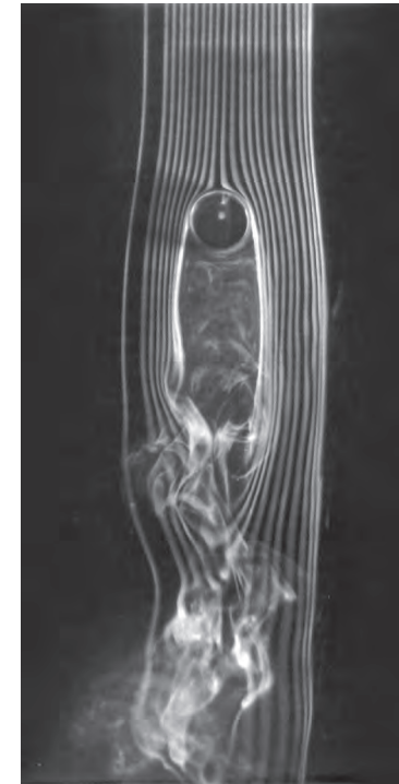
Figure 1. Marey's visualization for flow around a sphere.
