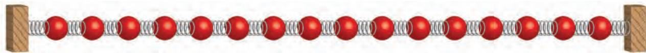
Figure 2. Lattice of masses coupled by nonlinear springs. The masses can move only in one dimension and the two ends of the chain were assumed to be fixed, i.e. u_0 = u_N = 0
